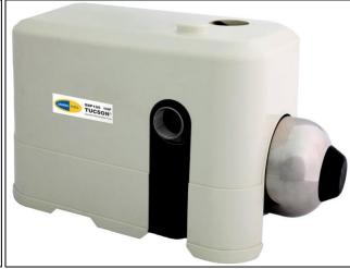
The **TUCSON®** SBP **Silent** Booster Pump series is an all-in-one automatic booster pump which combines motor, pump, accumulator, pressure & flow switch, all in one unit.
